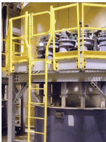
Raised platform with protected guardrail.
